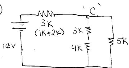
Find  $V_C$  first, Then do a Volt. Div. on  $3K, 4K$ . The  $3K, 4K$  are in series. ( $7K$ ). This result is in parallel with the  $5K$  ( $2.92K$ )
