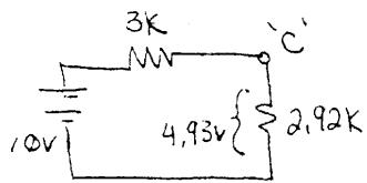
$$V_C = 10V \cdot \frac{2.92K}{3K+2.92K} = 4.93V \quad \text{This voltage divides between the original } 3K \text{ and } 4K.$$
