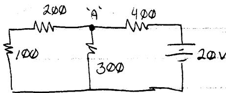
If we find  $V_A$ , we can get  $V_{200}$  from the voltage divider rule ( $200, 100$ ).
