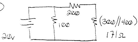
since the  $10\Omega$  is in parallel with the 20V source, it doesn't effect the voltage divider of  $200, 17.1$ .
