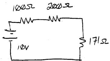
$V_{200}$  for this source is found via voltage divider rule:
