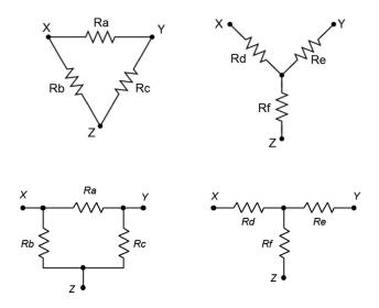
A true equivalent circuit would present the same resistance between any two terminals as the original circuit. For the unloaded case, we find:
