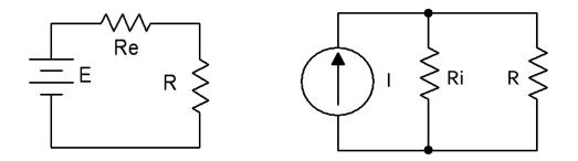
For equivalence, the load currents must be identical for both circuits given any value of load R. (Note that if the currents are the same then the voltages must also be the same due to Ohm's Law).
