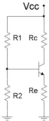
2. Plot the load line and determine  $V_E$ ,  $I_C$ ,  $V_C$ . Beta=200,  $R_E=3k$ ,  $R_C=1k$ ,  $R_E=2k$ ,  $V_{CC}=20V$ ,  $V_{EE}=-10.7V$
